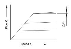
Max. flow deviation, Q max is 4.0 L/min Requirement of pilot oil for CPF  $\sim$  4.5 L/min. (max) Requirement of pilot oil for CPFR  $\sim$ 3 L/min. (max)
