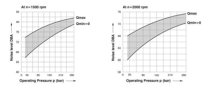
NOISE LEVEL VERSES OPERATING PRESSURE WITH FLUID ISO VG 46 DIN 51519 AT TEMP, t =  $50^{\circ}$ C Measuring error :  $\pm 2dB$  (A)
